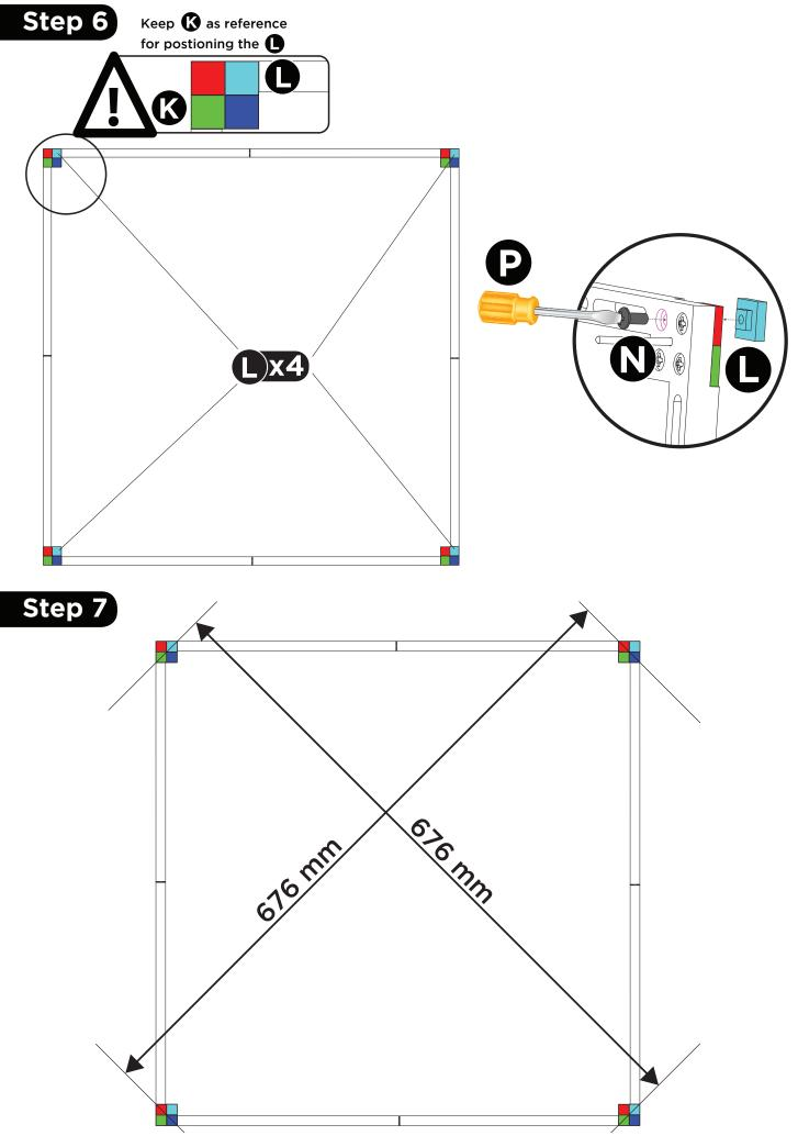
Keep in mind: when placing the reference on the bundle, all corners should have the red color at the top.
